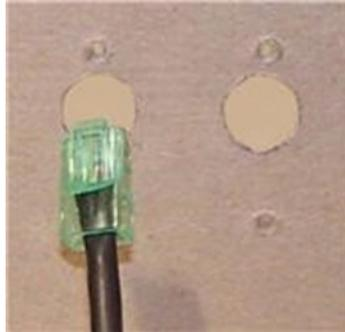
7. Align the four screws with the mounting holes and attach the ViVOpay Kiosk III to the outside surface. Ensure the cable is not pinched or binding.)
