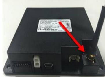
2. Attach the other end of the cable (80136204-001) from the antenna to the ViVOPay Kiosk III Controller.
