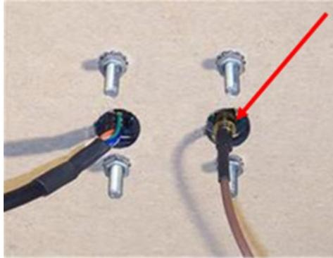
10. Attach the RJ45 connector coming from the ViVOPay Kiosk III Antenna to the RJ45 receptacle on the 80136204-001 cable.
