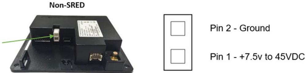
Connect +7.5 to 45VDC to the white two-socket Molex connector (mating connector Molex P/N 0039012020 with 5556-series crimps) or to pins 1 and 2 of the RS-232 connector (see next section).
