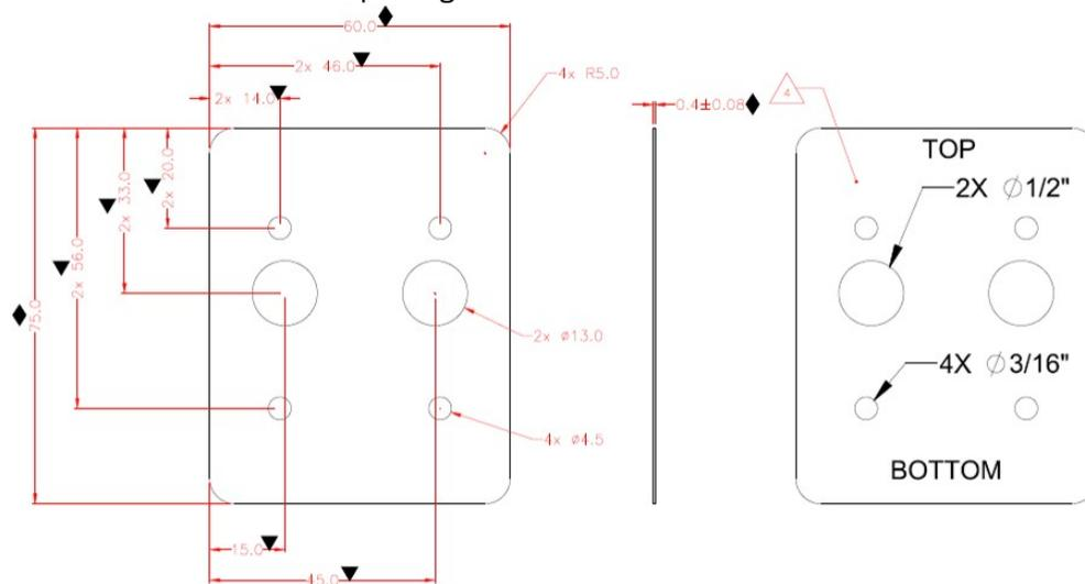
2. Locate and mark the two 14.0 mm (0.551 inches) access holes (used for connecting the antenna power, the LED power, and data cable to the ViVOpay Kiosk III).
