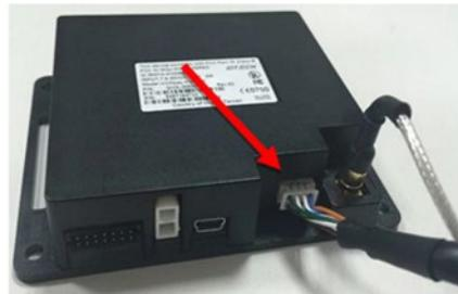
**Note:** Verify that the polarizing lug on the end of the data cable is facing towards the top of the ViVOPay Kiosk III Controller (away from the mounting plate) before inserting the cable. If the cable is installed incorrectly (upside down), it will apply the wrong polarity to the LEDs and damage them.
