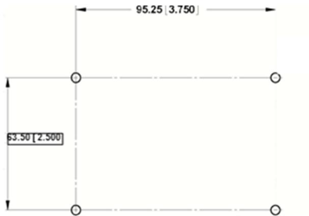
4. Drill the four 4.4 mm (0.173) mounting holes using a number 17 drill bit.
